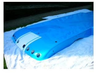
Parts were sent off to the soda blaster and then refurbished and powder coated. Parts that required complete replacement were drawn up and remanufactured, that included the whole of the aluminium bulkheads to the floor pan, I had these made by an aluminium fabrication specialist.
