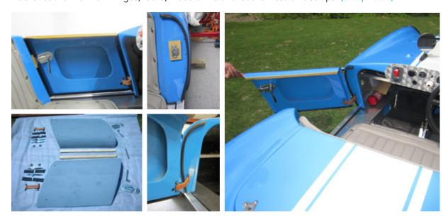
Rear seat cover rebuilt with cross brace strengthening bars and new locks fitted. (See photos)
