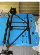
The next task was to rebuild all the wheel drums and braking components which were all new parts. Hand brake mechanism was rebuilt and fitted.
